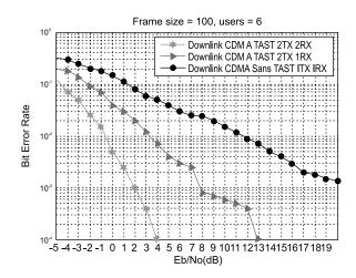
Figure 4. Performance analyses of DS-CDMA downlink channel with and without TAST code
