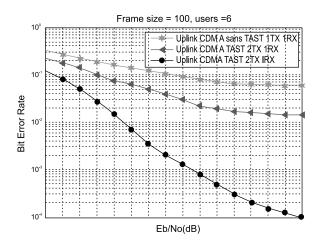
Figure 5. Performance analyses of DS-CDMA uplink channel with and without TAST codes
