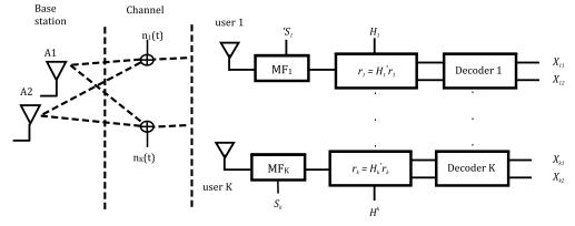
Figure 3. Downlink TAST CDMA receiver with one antenna
