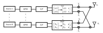
Figure 2. Uplink TAST CDMA transmitter with two transmit antenna
